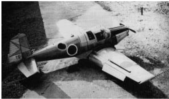
SAAB 91B TX-7101 X1G2, April, 1959 - Sep, 1960 Installed with gas turbine for providing compressed air to BLC blowing devices on leading and trailing edges of its wings.
