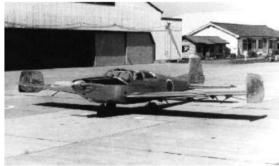
SAAB 91B TX-7101 X1G3, April, 1962 - Aug, 1962 Research for high lifting coefficient and lateral control by wing end plates.
